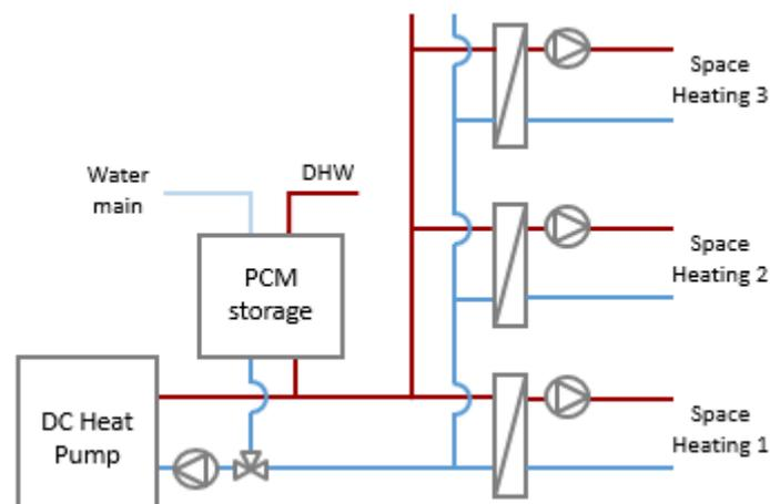
Figure 3. Scheme of Space Heating system with circuit isolating heat exchangers.
