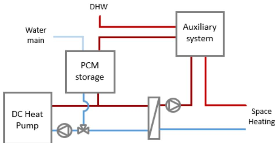
Figure 4. Scheme for the connection between the DC Heat Pump, the PCM storage and the auxiliary system.
