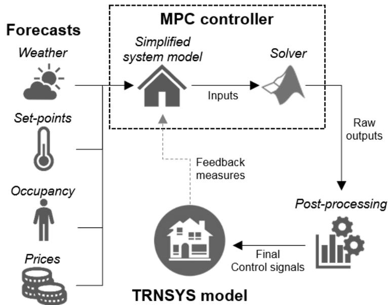
Figure 5. Scheme of the control system composed by the HRBC and MPC controllers [1].
